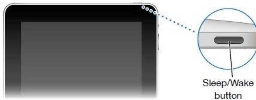
*Figure 1: The location of the Sleep/Wake button on the iPad is found at the upper right of the iPad with the glass side facing the user.*
